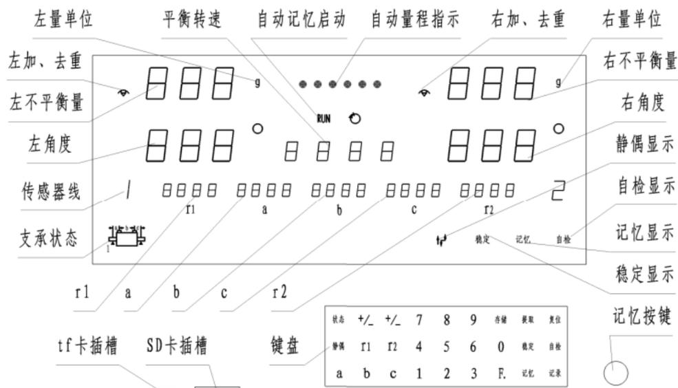
If you want to carry out the counterweight operation of couple unbalance, you should refer to Section 4.1 (dynamic balance method) to readjust the dimensions a, B and C after the static unbalance calibration is completed, and the static couple key will change the static couple state (dynamic balance correction method). In strict accordance with the (dynamic balance method) method, until the accuracy requirements.
